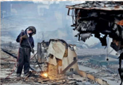
Breaking up of the Royal Navy ship HMS Fearless at the yard of Van Heyghen Recycling in Ghent, Belgium.
