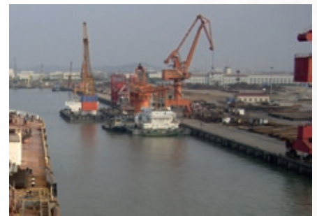
State-of-the-art shipbreaking yard in Jiangyin, China, with fixed and floating cranes.
